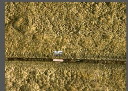
Weld Seam Corrosion Leak
