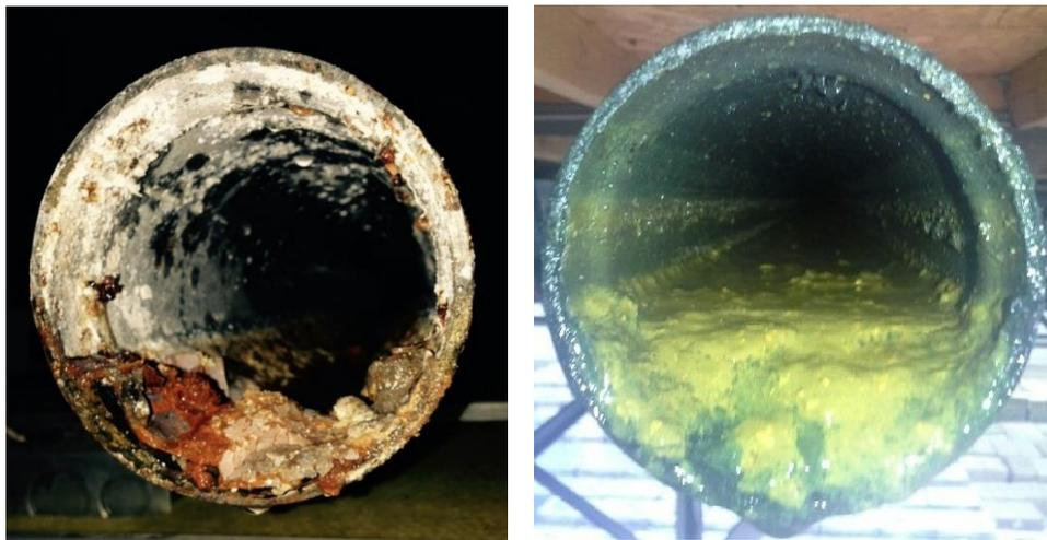
Left: galvanized pipe in dry system with trapped water
