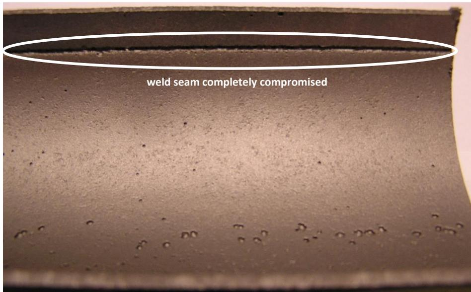
**Figure 2: Close-up of weld seam attack by acid corrosion**
