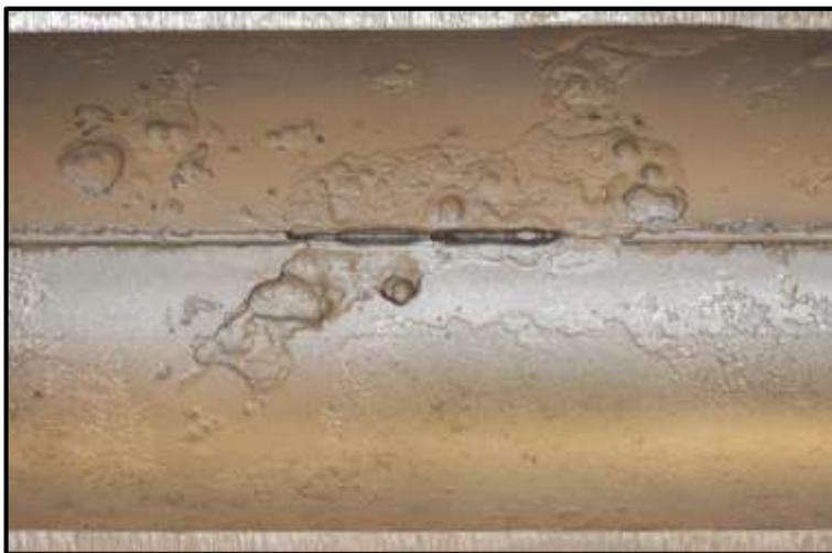
**Figure 4. Weld Seam Corrosion of 4" Galvanized Main**
