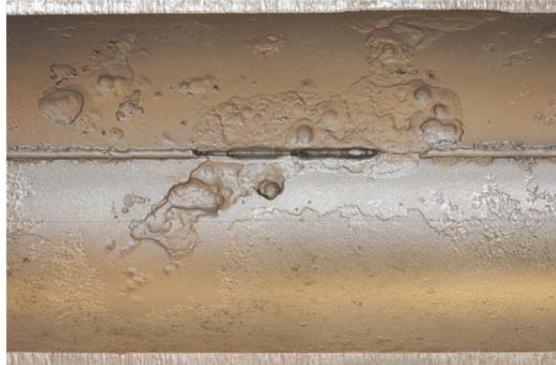
Knife cut corrosion on submerged weld seam
